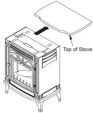
Figure 9 - Removing Top of Stove
